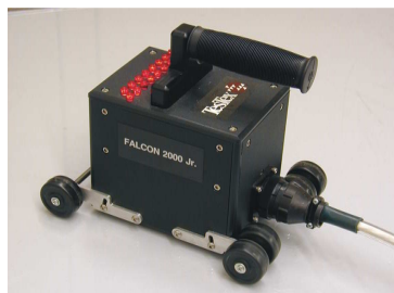
Falcon 2000 Jr. Hand Scanner used for Scanning hard to reach areas
