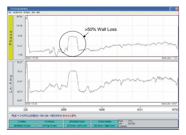
Above Waveform is of Row # 5, Tube # 4 showing Wall Loss > 50%.
